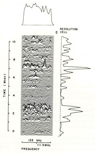
Narrowband spectra of individual subpulses. Each point of the intensity  $I_q(t)$  plotted on the right is the sum of the distribution of intensities across the receiver bandwidth shown in the center. At the top is plotted the spectrum averaged over the pulse. In the limit of many thousands of pulses this would show the receiver bandpass shape.
